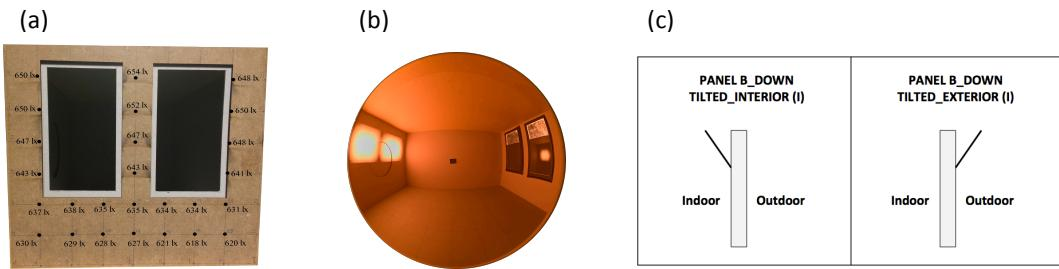
Figure 4. (a) Façade grid for taking vertical illuminance uniformity. (b) Rectangular black paper on a wall for taking Luminance measurement for further camera calibration (c) Tilted positions analysis
