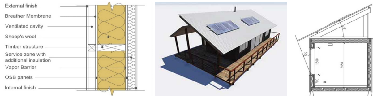
Fig. 4. Sectional detail of construction system. Fig. 5. Architectural application. Fig. 6 Section Physical test cell
